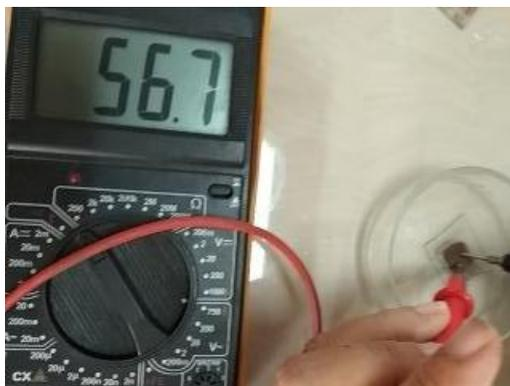
**Figure 4:** copper paste on glass substrate show the sheet resistance 56  $\Omega$
